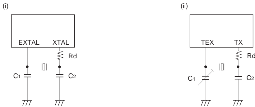
Fig. 13. Recommended oscillation circuit
